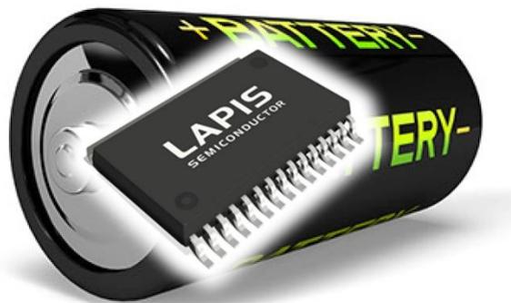
The [ML5245](#) is a standalone type that does not require control by a microcontroller. This has eliminated the need to develop specialized MCU
